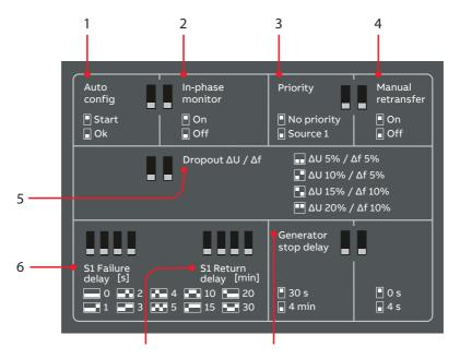
Fig. 4.1 DIP-switches for configuration in ZTX HMI
