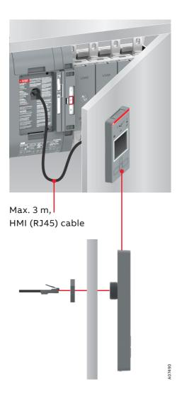
Fig. 9.4 HMI can be mounted on the switch or the door, door drilling. HMI protective cover available as accessory, type OXEC21, provides protection against accidental contact, see Chapter 10.3., Mounting of accessories
