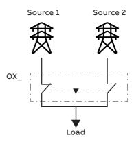
Fig. 2.3 Typical applications of automatic transfer switches
